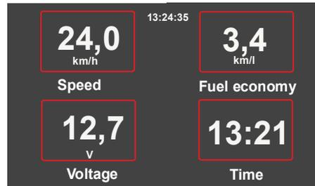
In the combi screen, parameters can be displayed using the increased character size for better readability. The parameters to be displayed are selected using the Settings button in the ZOOM Settings item.
