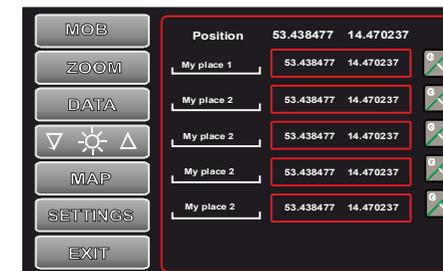
The screen above appears when MOB button is pressed. The position at the moment of pressing the button is saved and displayed at the top of the screen and can be saved in one of the 5 visible fields by holding this field for a few seconds. After saving, you can give it any name. If the name field is held down for a few seconds. Then a keyboard is displayed that allows you to enter any name of the item.
